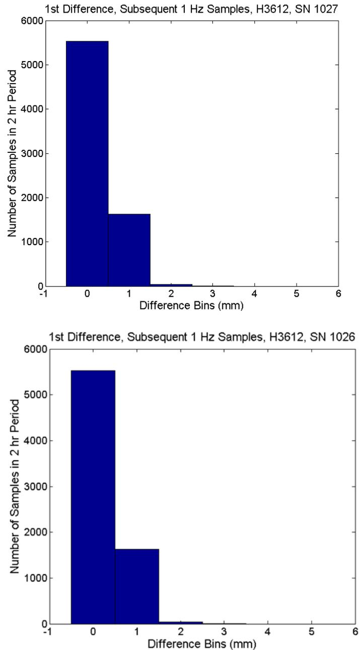
**Figure 3.** Histogram of first differences between subsequent 1-Hz range values shown in fig. 1, measured by H-3612.
