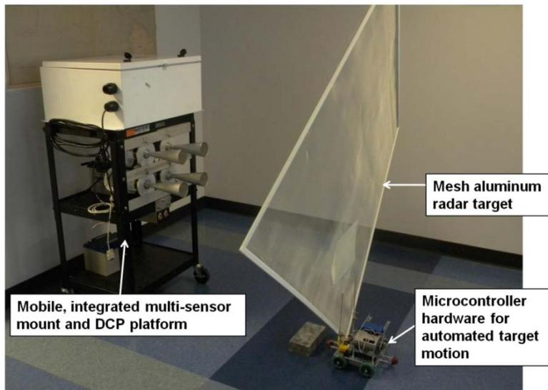
Figure 5. Example of radar time response test setup.
