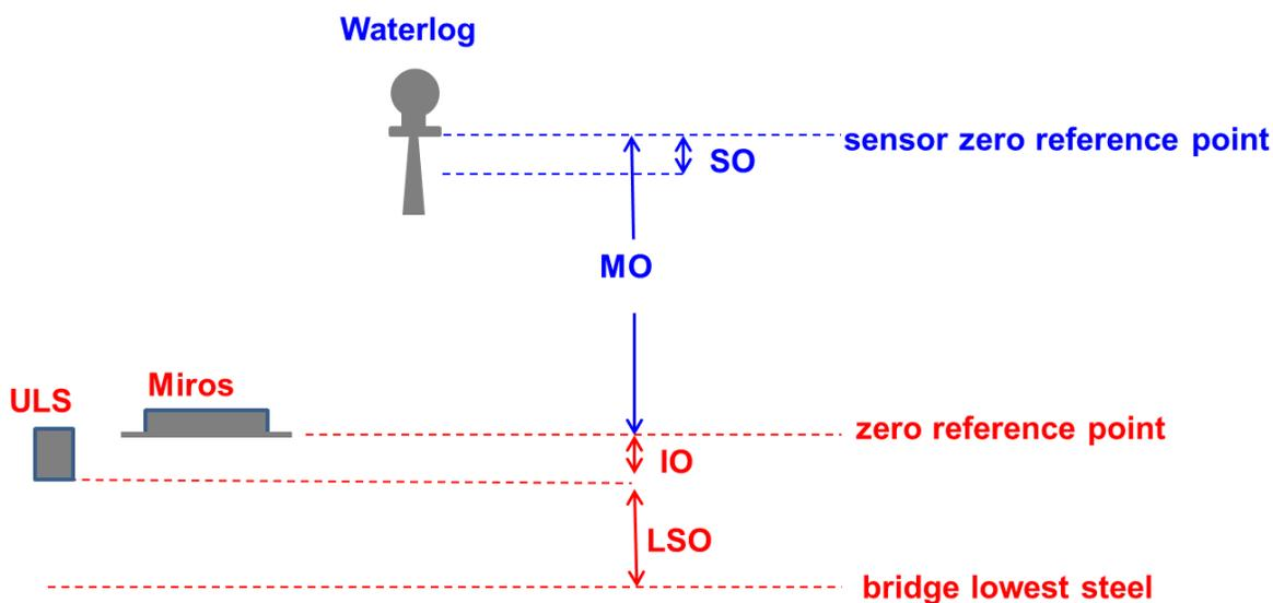
**Figure 22.** The set of vertical offsets that were applied to each sensor’s data records to vertically align range values before comparison.
