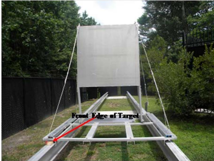
**Figure 8.** Metal target used during range verification laboratory test.
