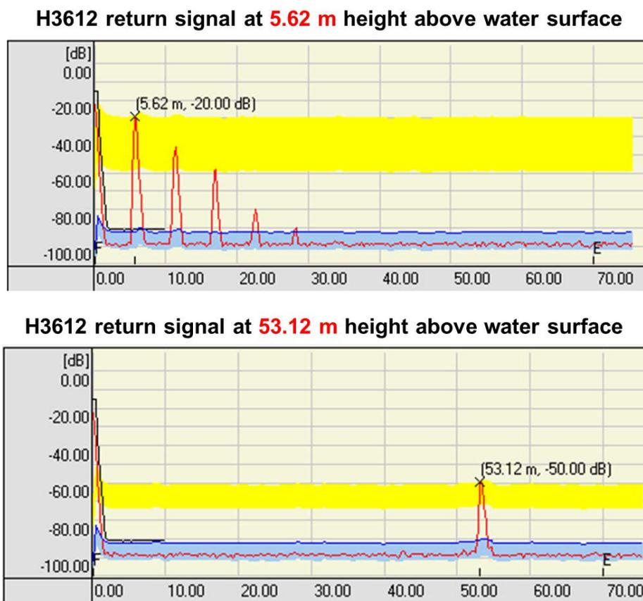
**Figure 15.** Return signals recorded by the WaterLog<sup>®</sup> H-3612 at the shortest (5.62 m) and longest (53.12 m) platform heights above the water surface during the crane lift test.
