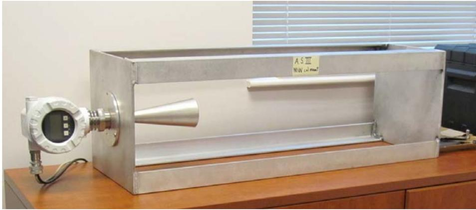
**Figure 4.** Sensor offset measurement mount designed at the Chesapeake Instrument Laboratory (CIL) by A. Sanford.
