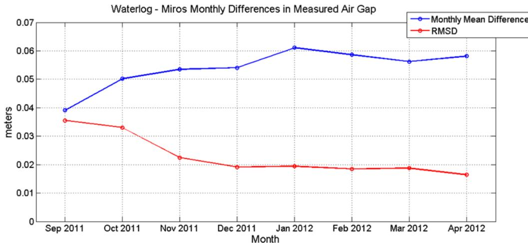
**Figure 30.** WaterLog<sup>®</sup> – Miros measured air gap differences; monthly mean differences (blue) and root mean squared deviation calculated after demeaning each sensors' records (red).
