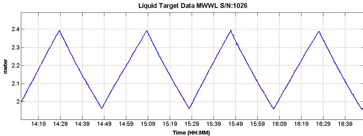
Figure 11. H3612 ranges measured during the liquid target test, while water levels in the test tank were gradually lowered and raised.
