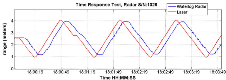
Figure 6. 1-Hz ranges measured by test WaterLog<sup>®</sup> H-3612 radar and reference ULS during the time response test.
