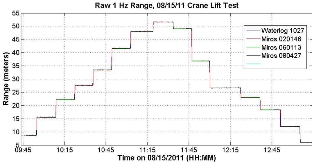
**Figure 13.** Time series of raw sensor-to-water surface range measured by the four sensors (three Miros and one test WaterLog<sup>®</sup> H-3612) during the 15 August 2011 over-water crane lift test.
