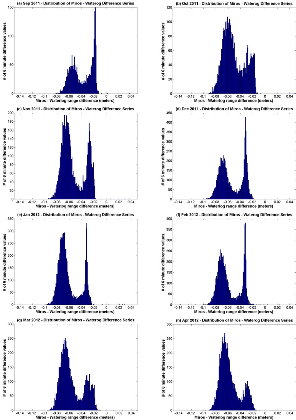
Figure 29. (a)- (h) Histograms created from each monthly difference series to show the distribution of sensors' 6-min range value differences.
