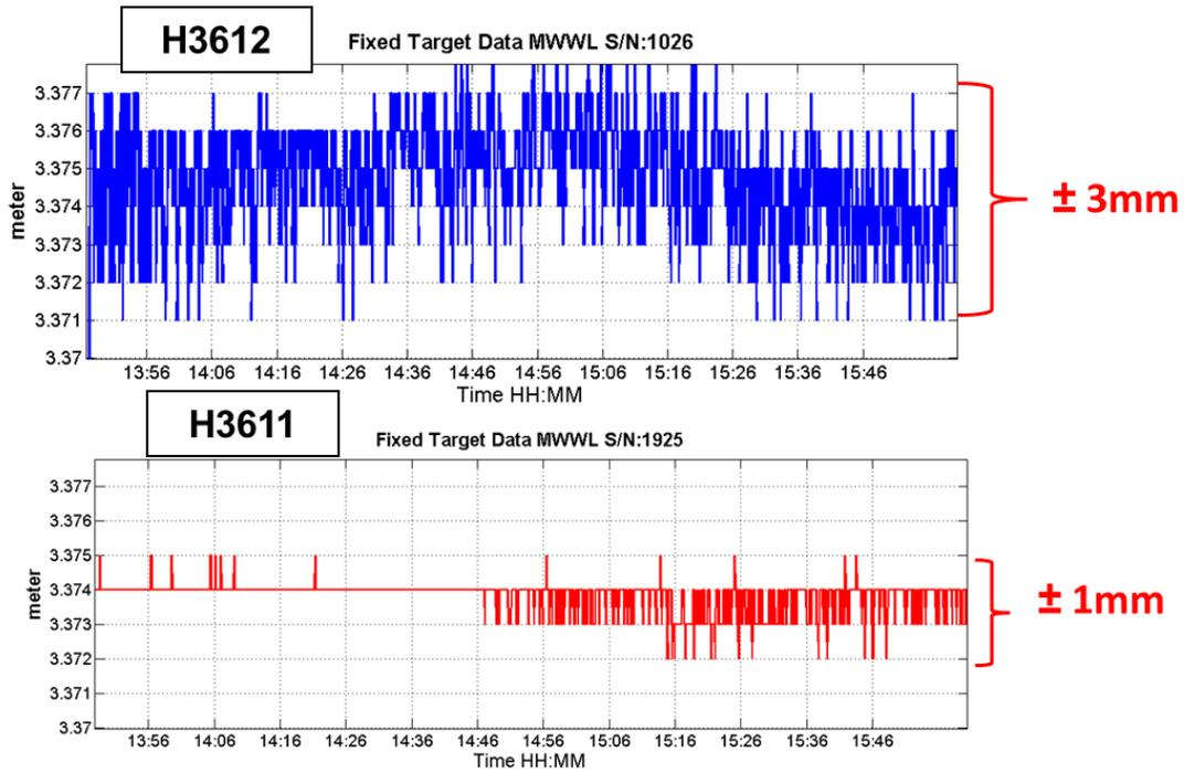
**Figure 1.** 1-Hz range time series collected during a fixed target lab test with a long range H-3612 (top) and a short range H-3611 (bottom).
