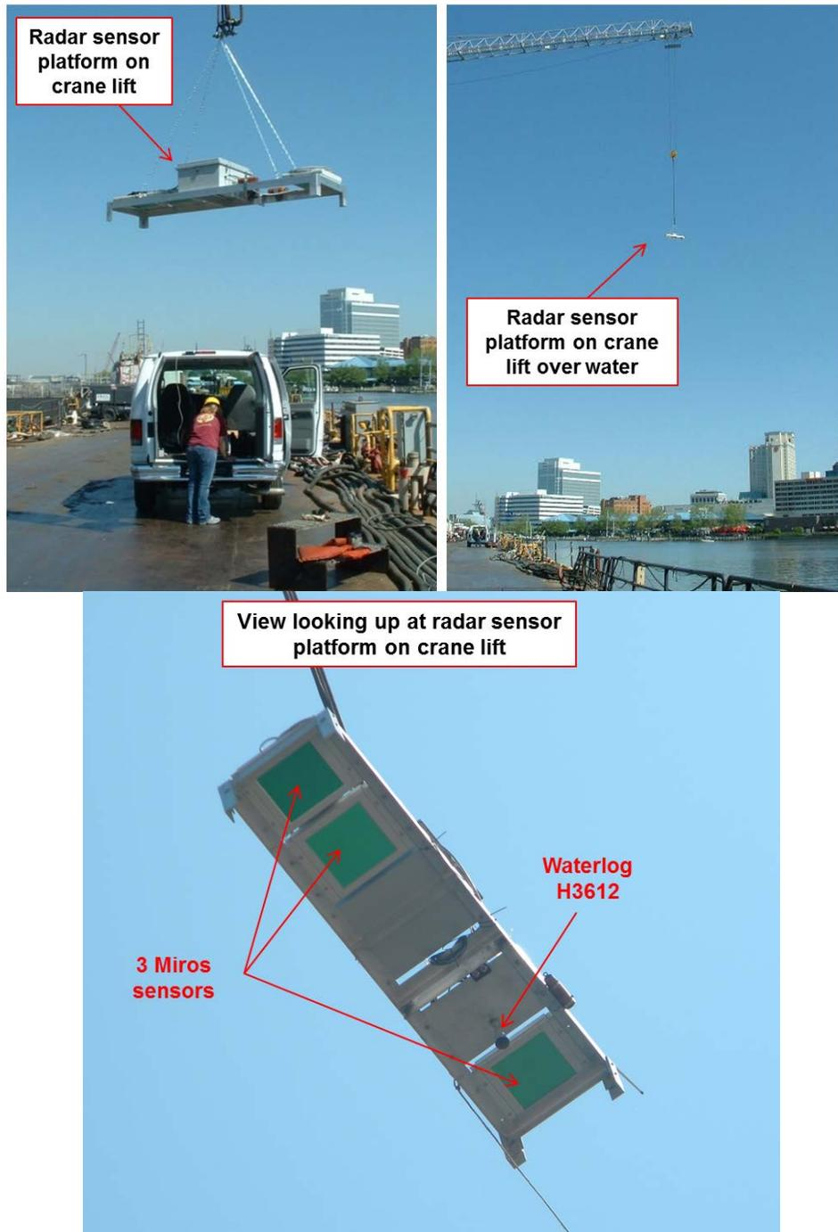
**Figure 12.** (a) Air gap sensor crane lift test platform at the Metro Machine facility along the Elizabeth River in Norfolk, VA. (b) View from below the crane-lifted sensor platform (looking upward) during the 15 August 2011, test.
