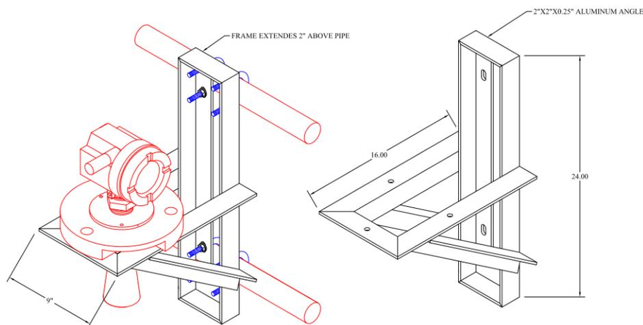
**Figure 18.** Conceptual drawing (by A. Sanford) of mount used to install the H-3612 test sensor on the bridge.
