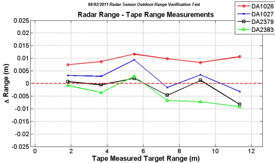
Figure 9. Results from range accuracy verification test.
