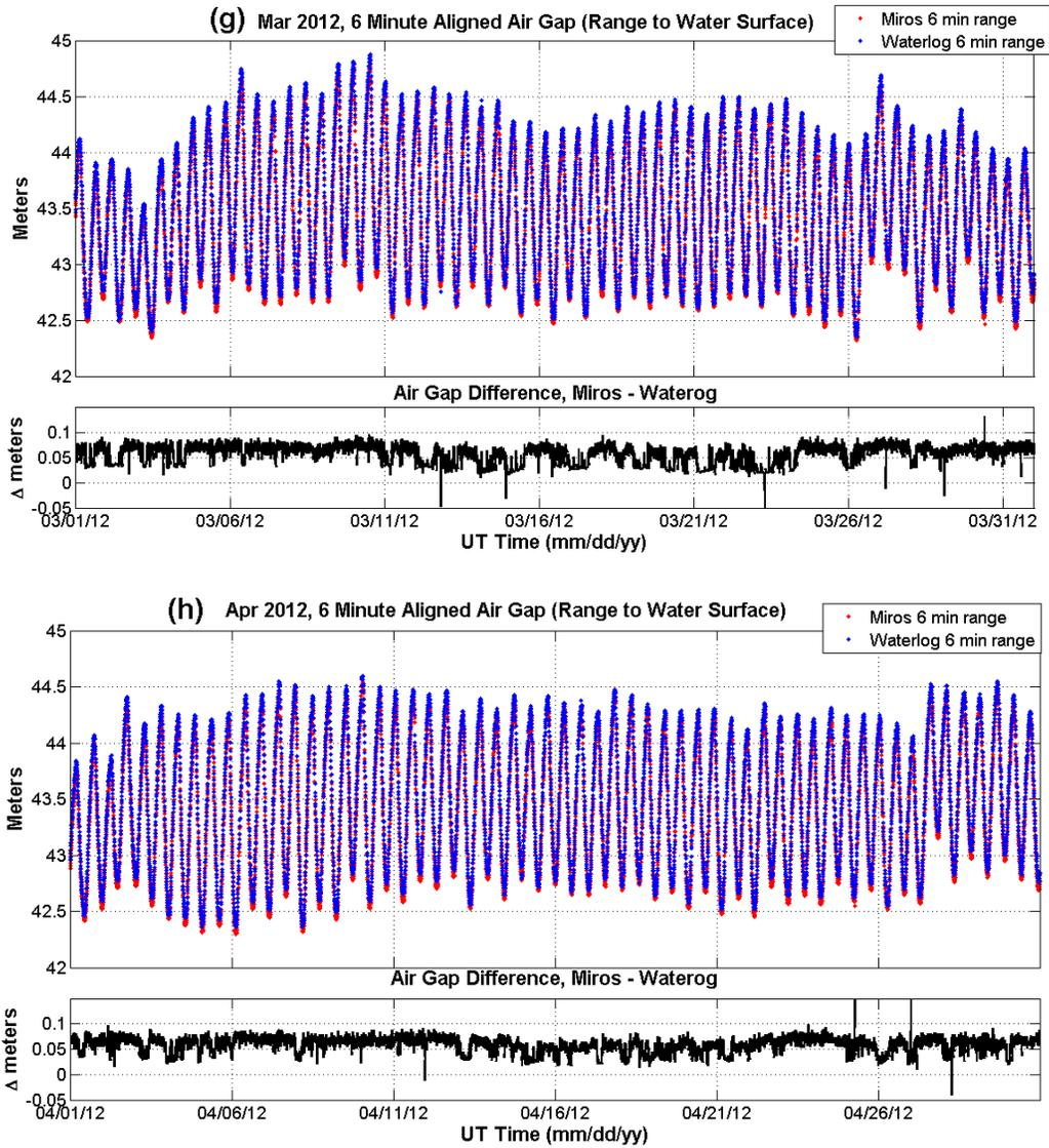
**Figure 28.** (a)-(h) September through April 2012 monthly time series plots of 6-min range series measured by the test WaterLog<sup>®</sup> radar and the operational Miros radar sensors (top panel) and the series of differences between the two sensors' measured ranges (bottom panel).
