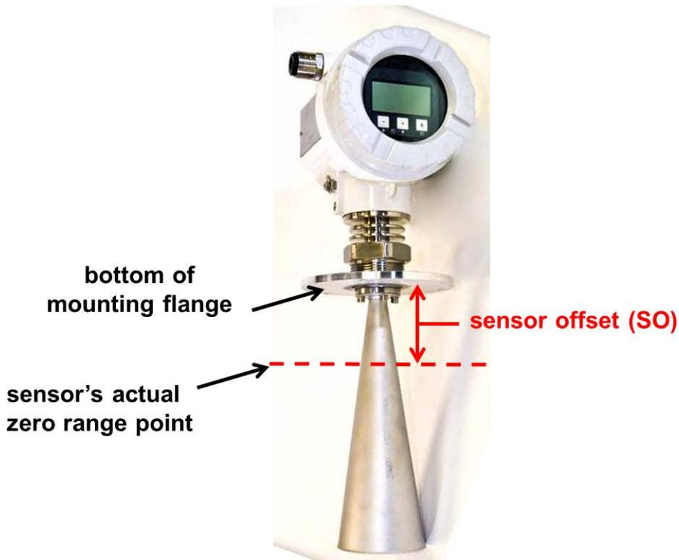
**NOTE: In example diagram shown here, sensor zero point is below the flange which will result in a positive sensor offset. In some cases, sensor zero point is above the flange which will result in a negative sensor offset**
