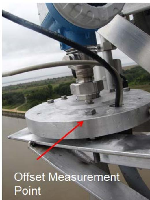
**Figure 20.** Test H-3612 radar sensor installed on bridge cage railing in mount with leveling collar.
