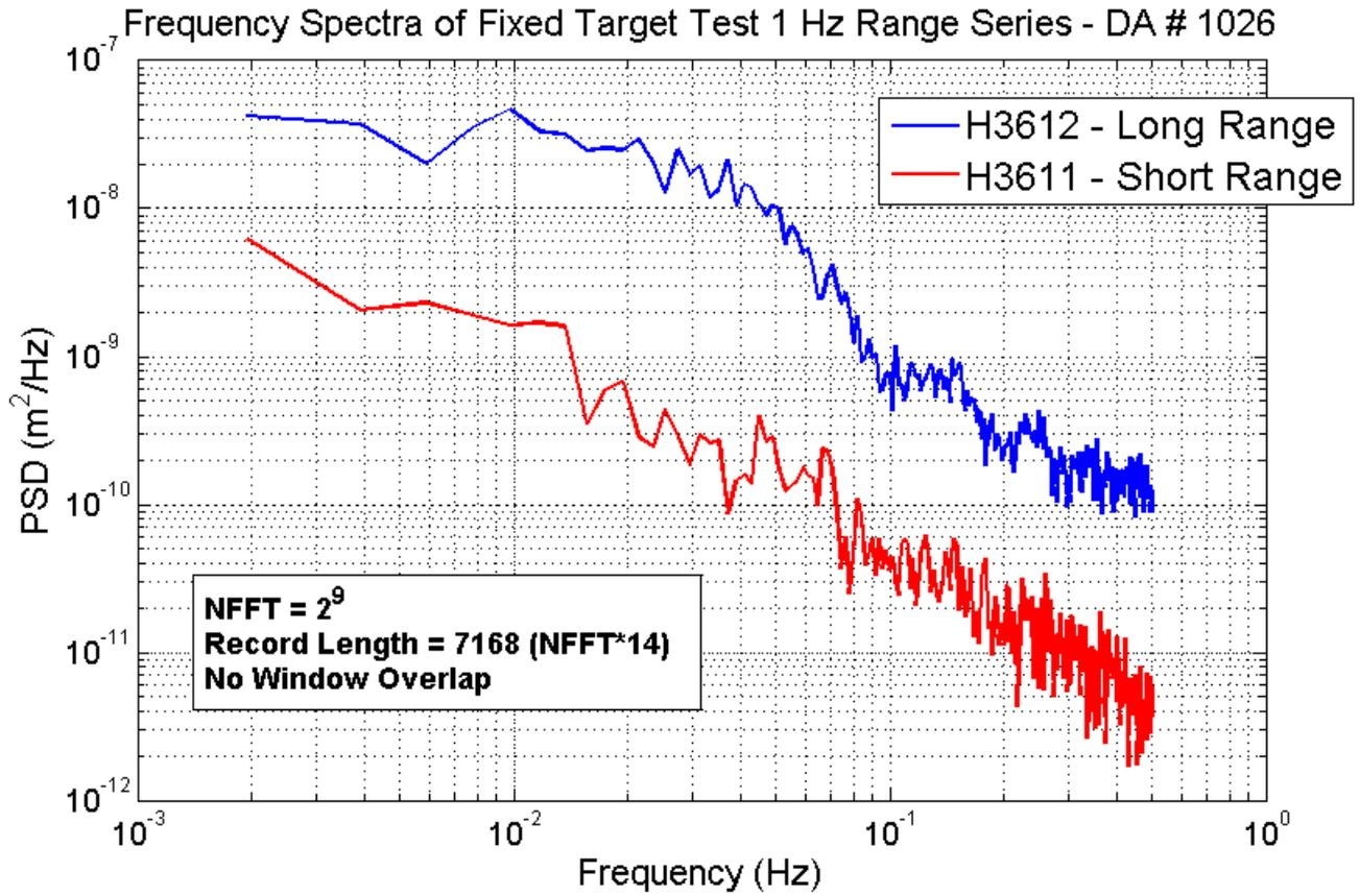
Figure 2. Frequency spectra calculated from the 1-Hz range time series shown in fig. 1.
