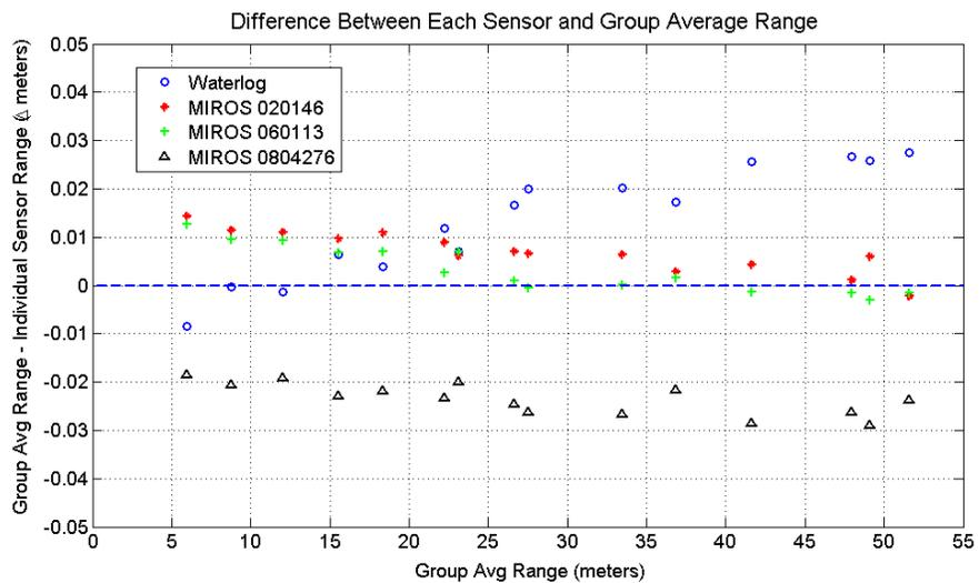
**Figure 14.** Difference between group average range calculated from all four radar sensors and individual sensors' range readings plotted against the group average range.
