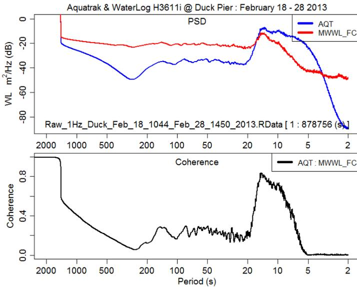
Figure 20. PSD and coherence of acoustic and microwave water level data at Duck, N.C. for February 18 - 28 2013.
