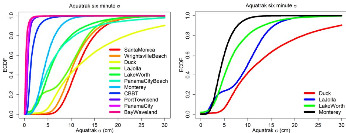
Figure 1. Empirical cumulative distribution functions of Aquatrak Data Quality and Assurance Procedure (DQAP)  $\sigma$  over a period of 1 year at coastal NWLON stations (left). Empirical cumulative distribution functions of Aquatrak DQAP  $\sigma$  over a period of 1 year at four NWLON stations selected for Phase II analysis (right).
