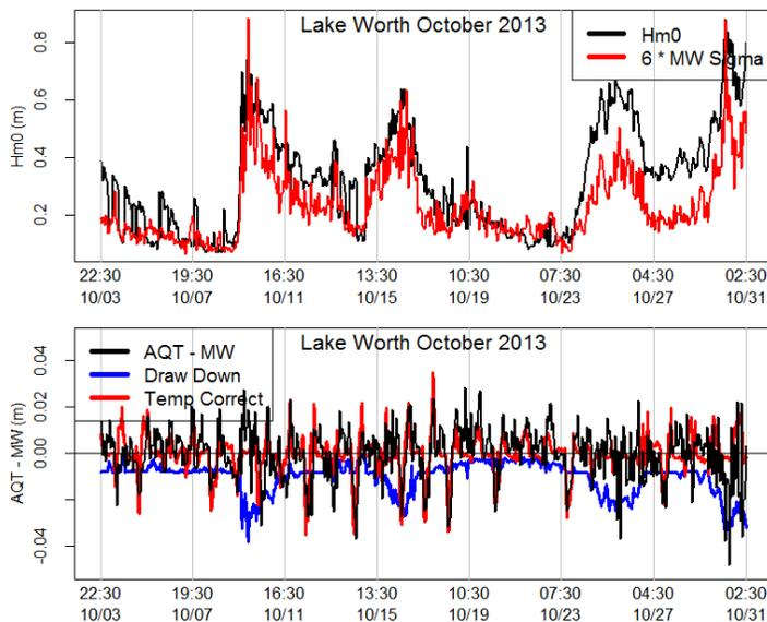
Figure 35. Significant wave height and microwave DQAP standard deviation (top) at Lake Worth in October 2013. Water level difference (acoustic - microwave) with acoustic temperature and wave draw-down corrections (bottom).
