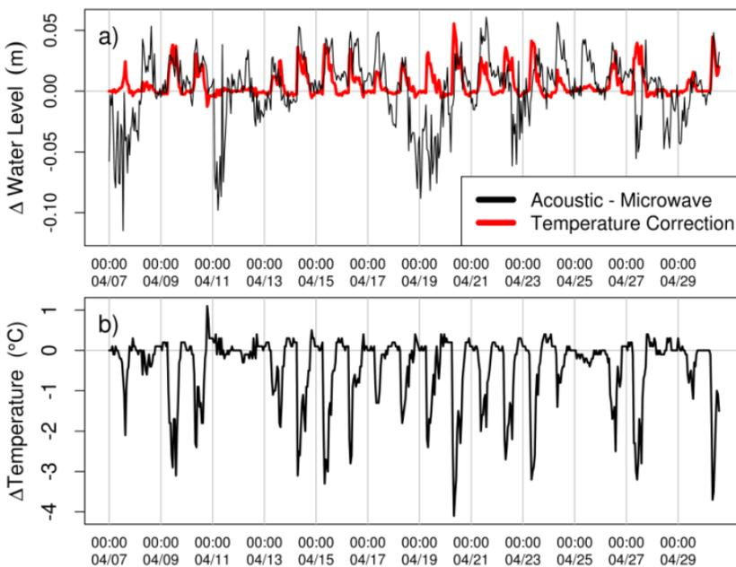
Figure 9. Hourly data and temperature corrections from Duck in April 2012. a) Water level difference between the acoustic and microwave sensors (black) and acoustic temperature water level error estimates (red). b) Temperature difference between the upper and lower thermistors of the acoustic sounding tube.
