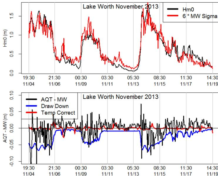
Figure 37. Significant wave height and microwave DQAP standard deviation (top) at Lake Worth in November 2013. Water level difference (acoustic - microwave) with acoustic temperature and wave draw-down corrections (bottom).
