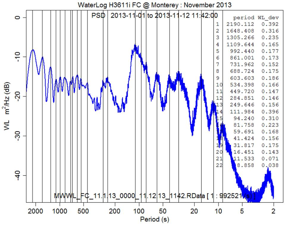
Figure 45. PSD estimate of microwave water level at Monterey for November 1 - 12, 2013. Vertical lines mark frequencies of interest. The inset table lists the period of oscillation in seconds for each vertical line and the corresponding water level oscillation amplitude in meters.
