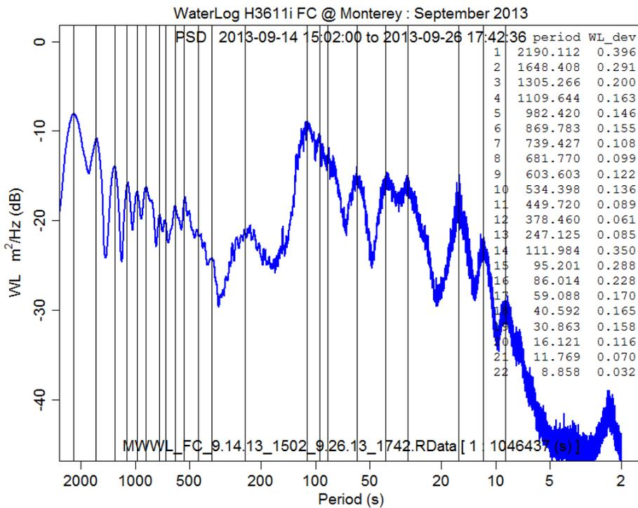
Figure 39. PSD estimate of microwave water level at Monterey for September 14 - 26, 2013. Vertical lines mark frequencies of interest. The inset table lists the period of oscillation in seconds for each vertical line and the corresponding water level oscillation amplitude in meters.
