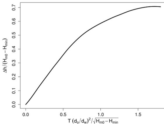
Figure 5. Relationship between water level draw-down in centimeters ( $\Delta h$ ) and surface wave forcing.  $T$  is the wave period,  $d_o/d_w$  the ratio of orifice to protective well diameter,  $H_{m0}$  the significant wave height in meters, and  $H_{min}$  a minimum threshold wave height below which wave effects are not important.
