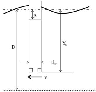
Figure 4. Schematic of protective well orifice with a hydraulic current of velocity  $v$  across the orifice.
