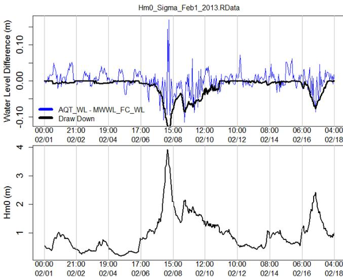
Figure 19. Water level difference (acoustic - microwave, blue) and water level draw-down estimate (black) and significant wave height at Duck, N.C. for February 1 - 18 2013.
