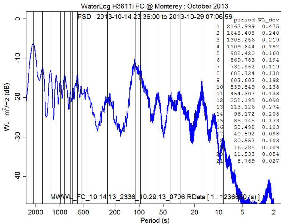
Figure 43. PSD estimate of microwave water level at Monterey for October 14 - 29, 2013. Vertical lines mark frequencies of interest. The inset table lists the period of oscillation in seconds for each vertical line and the corresponding water level oscillation amplitude in meters.
