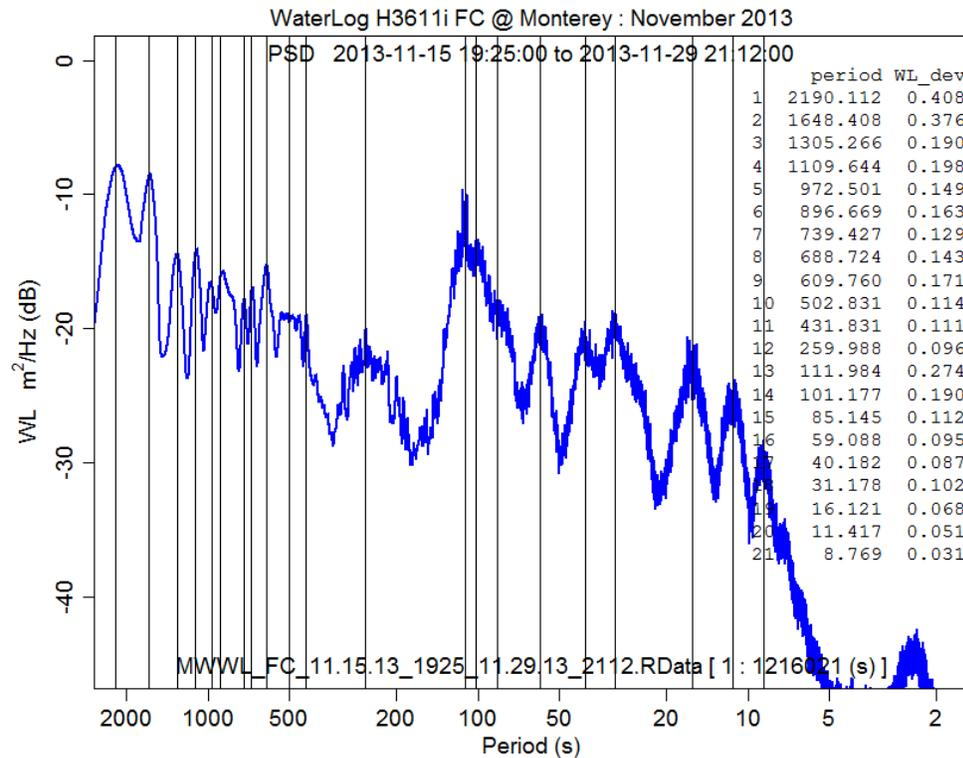
Figure 47. PSD estimate of microwave water level at Monterey for November 15 - 29, 2013. Vertical lines mark frequencies of interest. The inset table lists the period of oscillation in seconds for each vertical line and the corresponding water level oscillation amplitude in meters.
