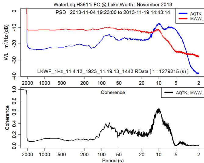
Figure 36. PSD and coherence of acoustic and microwave water level data at Lake Worth for November 2013.
