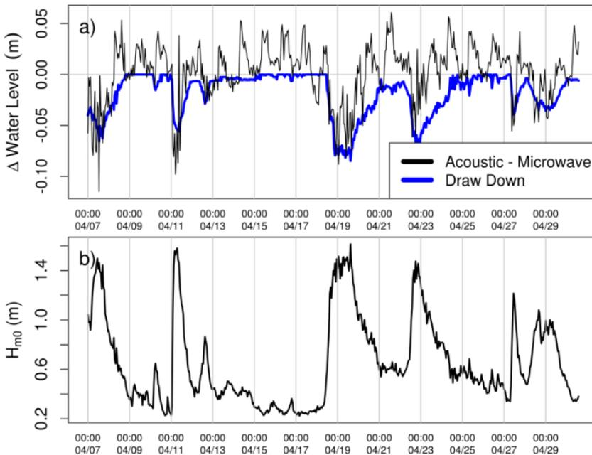
Figure 10. Hourly data and draw-down corrections from Duck in April 2012. a) Water level difference between the acoustic and microwave sensors (black) and protective well draw-down estimates (blue). b) Significant wave height.
