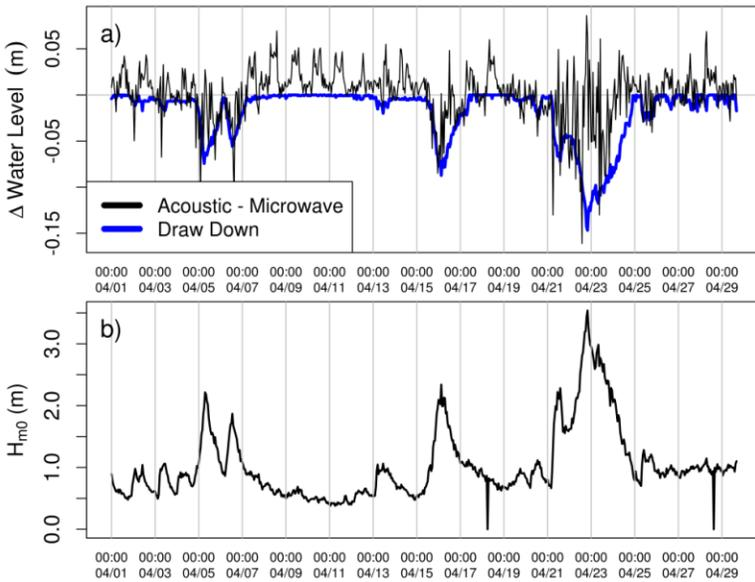
Figure 24. Hourly data and draw-down corrections from Duck N.C. in April 2013. a) Water level difference between the acoustic and microwave sensors (black) and protective well draw-down estimates (blue). b) Significant wave height.
