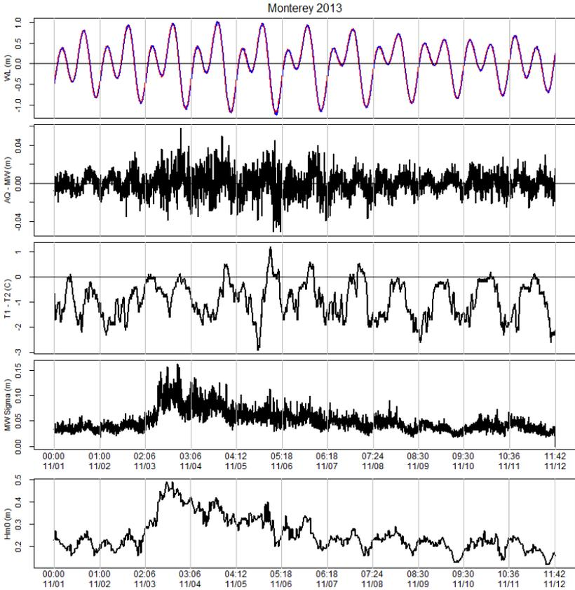
Figure 44. Monterey data for November 1 - 12, 2013. WL is the demeaned DQAP water level, microwave data are red, acoustic data are blue. AQ - MW is the water level difference. T1 - T2 is the temperature difference of the two thermistors. MW Sigma is the DQAP standard deviation ( $\sigma$ ) of the microwave data.  $H_{m0}$  is the significant wave height.
