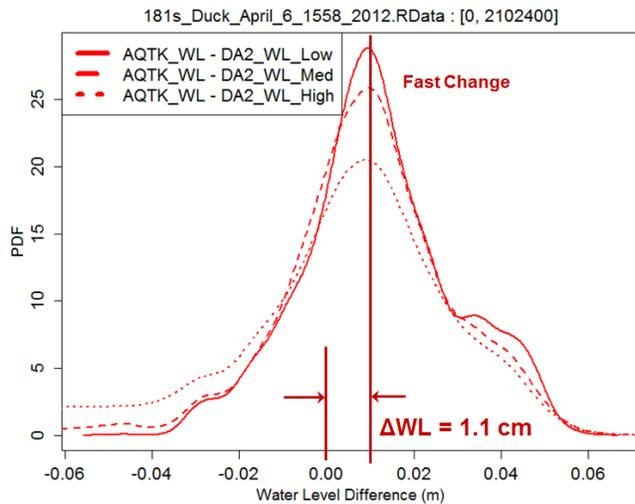
Figure 11. Probability density functions of range to water difference (acoustic - microwave) for April 2012 at Duck. Density functions are shown for: Low ( $0 < \sigma < 1/3$ ), Medium ( $1/3 < \sigma < 2/3$ ), and High ( $\sigma > 2/3$ ) partitions of the data.
