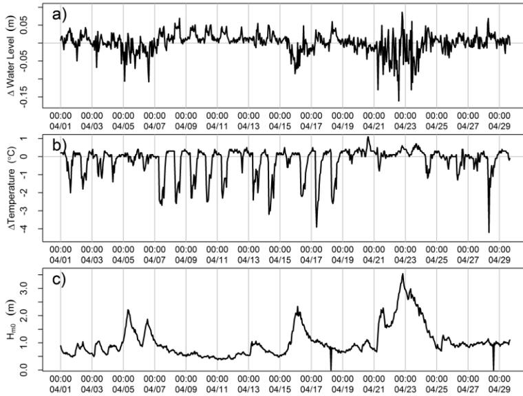
Figure 22. Hourly data from Duck, N.C. in April 2013. a) Water level difference between the acoustic and microwave sensors. b) Temperature difference between the upper and lower thermistors of the acoustic sounding tube. c) Significant wave height.
