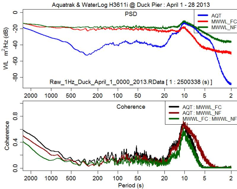
Figure 26. PSD and coherence of acoustic and microwave water level data at Duck NC for April 2013.
