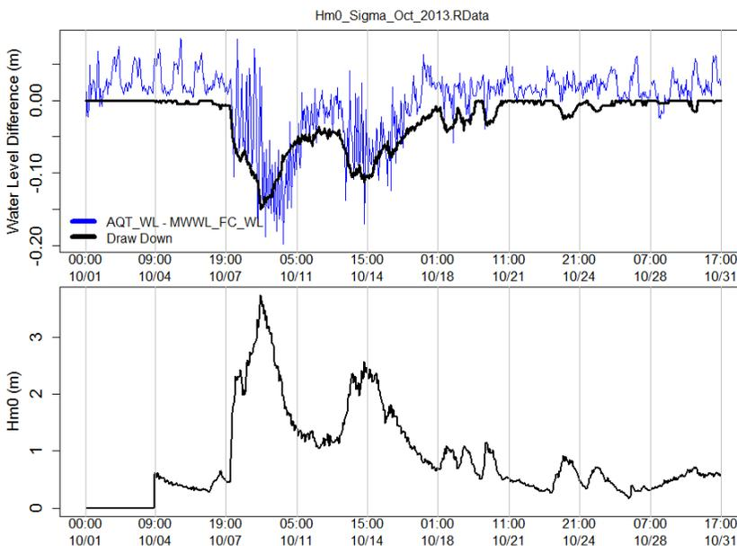
Figure 27. Hourly data and draw-down corrections from Duck, North Carolina in April 2013. a) Water level difference between the acoustic and microwave sensors (blue) and protective well draw-down estimates (black). b) Significant wave height.
