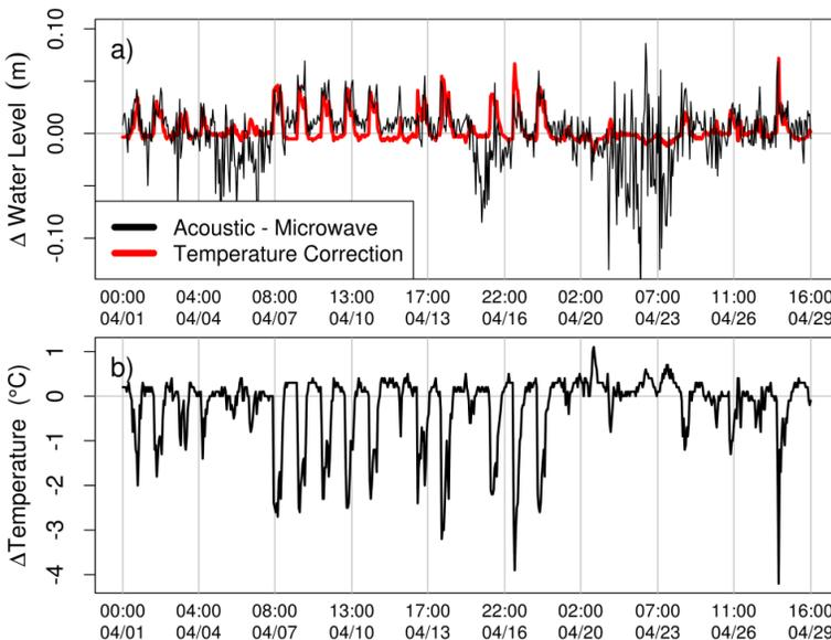
Figure 23. Hourly data and temperature corrections from Duck, N.C. in April 2013. a) Water level difference between the acoustic and microwave sensors (black) and acoustic temperature water level change estimates (red). b) Temperature difference between the upper and lower thermistors of the acoustic sounding tube.
