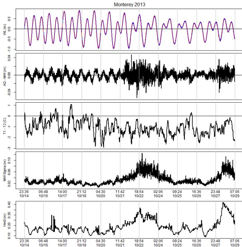
Figure 42. Monterey data for October 14 - 29, 2013. WL is the demeaned DQAP water level, microwave data are red, acoustic data are blue. AQ - MW is the water level difference. T1 - T2 is the temperature difference of the two thermistors. MW Sigma is the DQAP standard deviation ( $\sigma$ ) of the microwave data.  $H_{m0}$  is the significant wave height.
