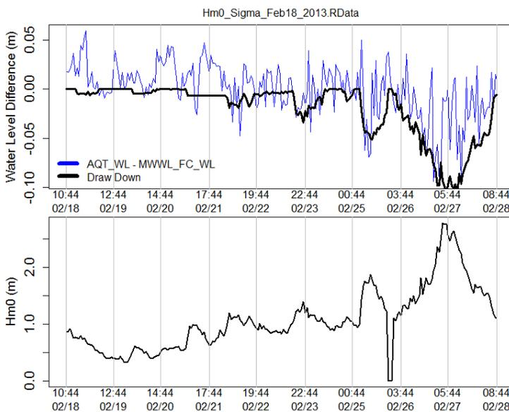
Figure 21. Water level difference (acoustic - microwave, blue) and water level draw-down estimate (black) and significant wave height at Duck, N.C. for February 18 - 28 2013.
