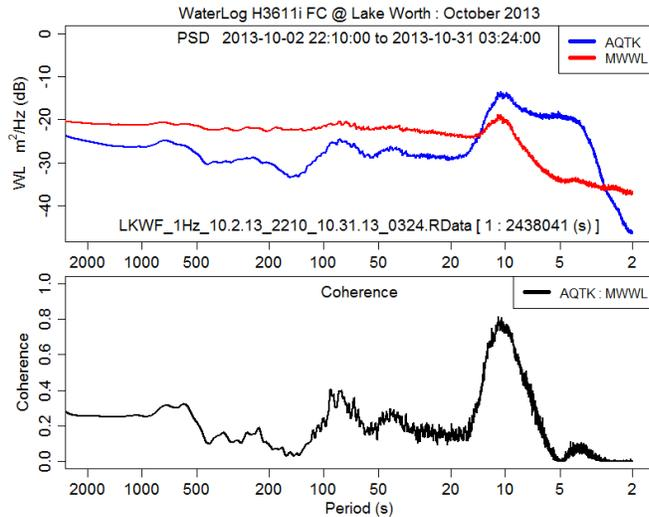
Figure 34. PSD and coherence of acoustic and microwave water level data at Lake Worth for October 2013.
