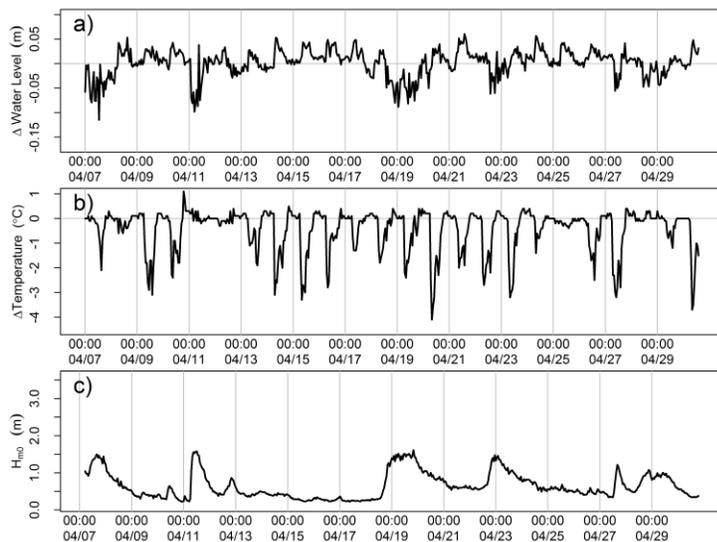
Figure 6. Hourly data from Duck, N.C. in April 2012. a) Water level difference between the acoustic and microwave sensors. b) Temperature difference between the upper and lower thermistors of the acoustic sounding tube. c) Significant wave height. Times are Coordinated Universal Time (UTC).
