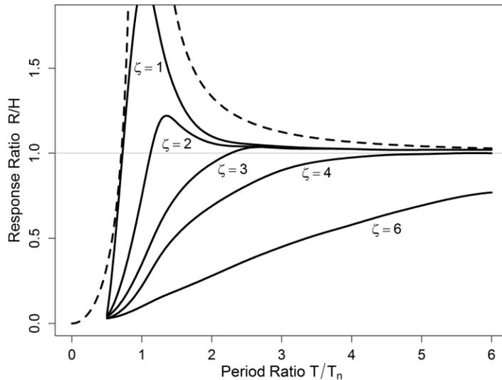
Figure 3. Dynamic water level response inside a protective well to surface waves of height  $H$  and period  $T$ .  $R$  is the water level amplitude,  $T_n$  is the resonant period of the well and  $\zeta = d_w/d_o$  is the damping factor where  $d_w$  and  $d_o$  are the diameters of the protective well and orifice, respectively. The dashed line represents the theoretical response in the absence of damping.
