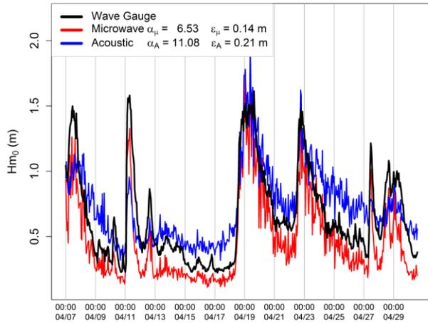
Figure 14. Hourly significant wave height ( $H_{m0}$ ) and estimates of wave height ( $\hat{H}_{m0}$ ) from a linear model of  $H_{m0}$  regressed onto water level standard deviations ( $\sigma$ ) over 24 days of April 2012 at Duck.  $\alpha$  is the fit coefficient,  $\varepsilon$  the RMS residual between wave gauge  $H_{m0}$  and estimated wave height ( $\hat{H}_{m0}$ ).
