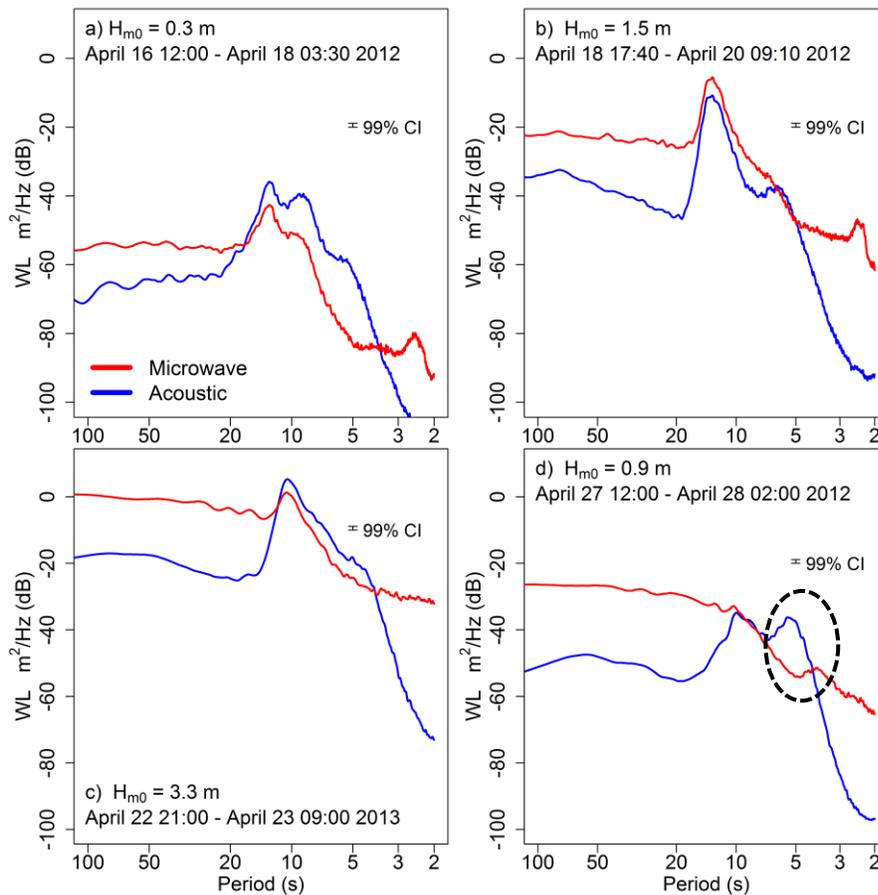
Figure 7. Power spectral density estimates of 1 Hz water level data from the acoustic and microwave sensors at Duck, N.C. a) Low wave conditions. b) Intermediate to high wave conditions. c) Very high wave conditions. d) A locally generated, short duration swell with a dominant period of 4.1 seconds. Spectral distortion from the well resonance is highlighted.
