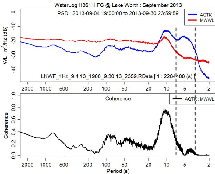
Figure 8. PSD of 1 Hz water level data from Lake Worth during September 2013. Resonance of the protective well is presented as a large distortion of the spectral variance centered on a period of 5 seconds. The lack of coherence between the acoustic and microwave water levels at 5 seconds indicates that this resonant energy is a distortion.
