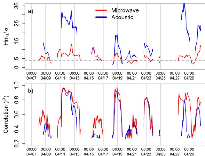
Figure 15. Linear regression of significant wave height ( $H_{m0}$ ) onto microwave and acoustic standard deviations shown in Figure 13 over a 24-hour sliding window. a) Fit coefficients. The dashed line shows the ideal model of  $H_{m0} = 4\sigma$ , corresponding to the accepted definition of significant wave height. b) Correlation coefficients. Values are shown only if the p-value exceeded the 99% significance level.
