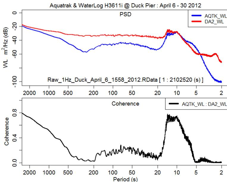
Figure 17. PSD and coherence of acoustic and microwave water level data at Duck, N.C. in April 2012.
