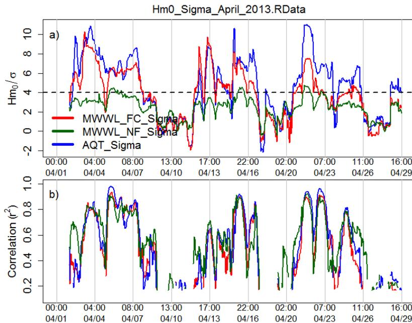
Figure 16. Linear regression of DQAP  $\sigma$  and significant wave height for the acoustic and microwave sensors during April 2013. a) Fit coefficients b) Correlation coefficient. Values are shown only if the p-value exceeded the 95% confidence interval. The dashed line shows the canonical definition of  $H_{m0} = 4 \sigma$ .
