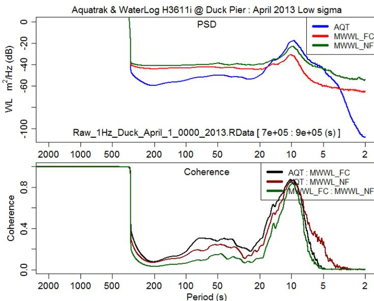
Figure 25. PSD and coherence of acoustic and microwave water level data at Duck, N.C. for April 9 - 11, 2013, a period of low surface energy.
