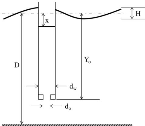
Figure 2. Schematic diagram of Aquatrak protective well. The water depth is  $D$ , the instantaneous water level from the mean is  $x$ , submergence depth  $Y_o$ , well diameter  $d_w$ , orifice diameter  $d_o$  and wave amplitude  $H$ .
