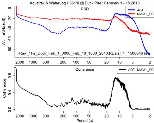
Figure 18. PSD and coherence of acoustic and microwave water level data at Duck, N.C. for February 1 - 18 2013.
