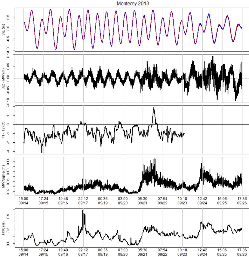
Figure 38. Monterey data for September 14 - 26, 2013. WL is the demeaned DQAP water level, microwave data are red, acoustic data are blue. AQ - MW is the water level difference. T1 - T2 is the temperature difference of the two thermistors. MW Sigma is the DQAP standard deviation ( $\sigma$ ) of the microwave data. Hm0 is the significant wave height.
