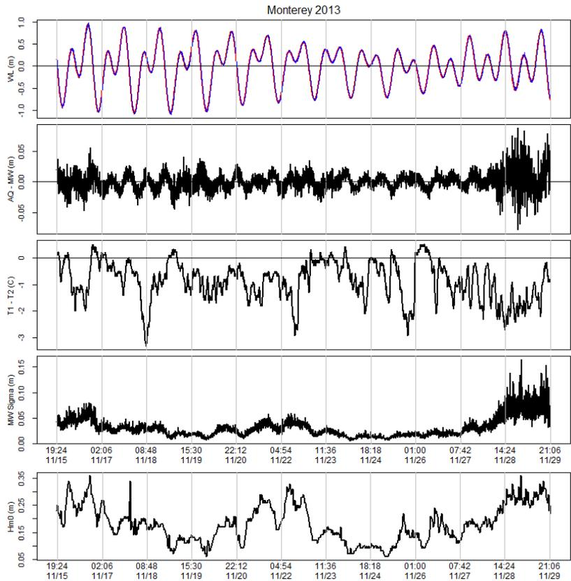
Figure 46. Monterey data for November 15 - 29, 2013. WL is the demeaned DQAP water level, microwave data are red, acoustic data are blue. AQ - MW is the water level difference. T1 - T2 is the temperature difference of the two thermistors. MW Sigma is the DQAP standard deviation ( $\sigma$ ) of the microwave data.  $H_{m0}$  is the significant wave height.
