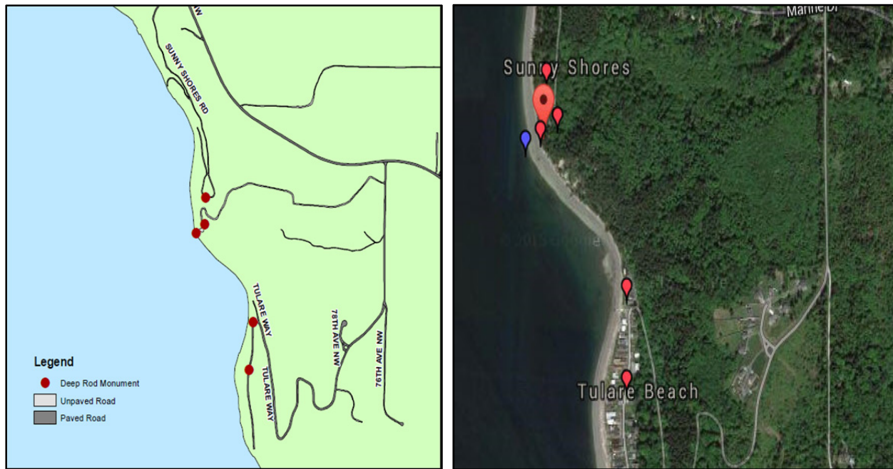
Figure 14. Locations of deep rod marks at Tulare Beach, WA (left). Graphic courtesy of Dorrel Dickson. Locations of full tidal bench mark network (right) for Tulare Beach, WA. The large red balloon identifies the water level station location. The small red balloons identify published tidal bench marks and the blue balloon identifies an unpublished tidal bench mark.
