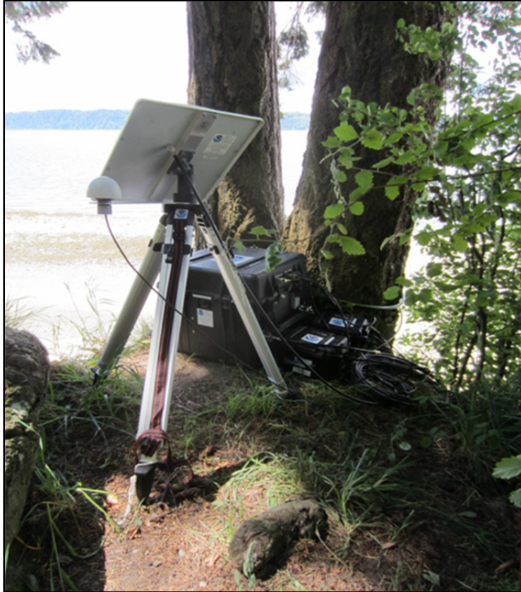
Figure 3. Portable Data Collection Platform (DCP), flat panel GOES antenna, and GPS antenna at Tulare Beach, WA.
