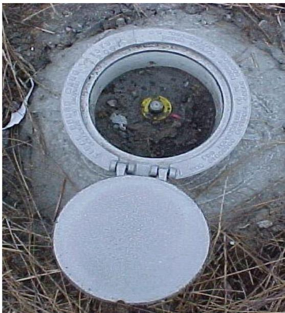
**Figure 7.** Tidal bench mark with capped PVC flanged noted as 8571579 A TIDAL.
