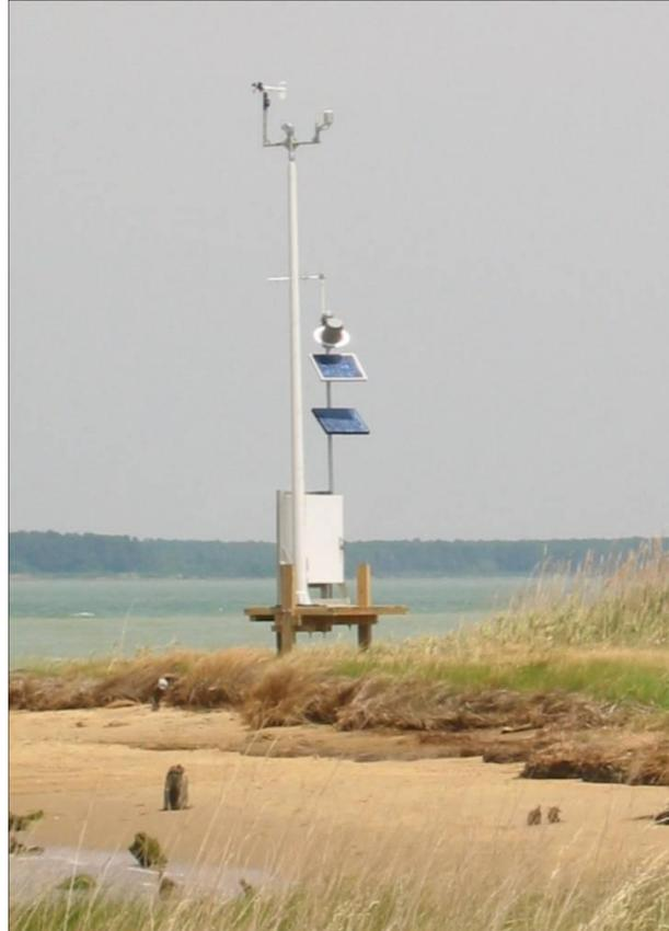
**Figure 3.** Barren Island water level station featuring GOES antenna, solar panels, barometer, and wind sensor (anemometer).
