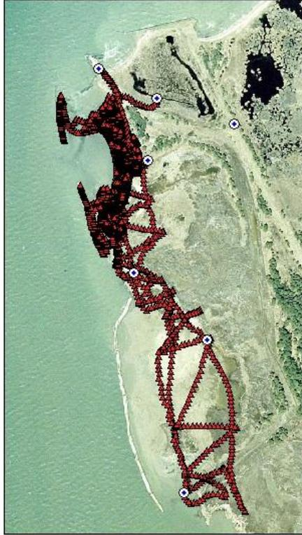
**Figure 9.** Kinematic GPS data overlaid on aerial photography of Barren Island.
