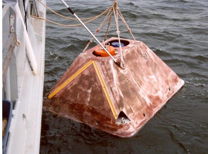
**Figure 5.** The bottom-mounted ADCP transducer head (in blue) can be seen as it is lowered to the Chesapeake Bay floor for waves and current data collection.
