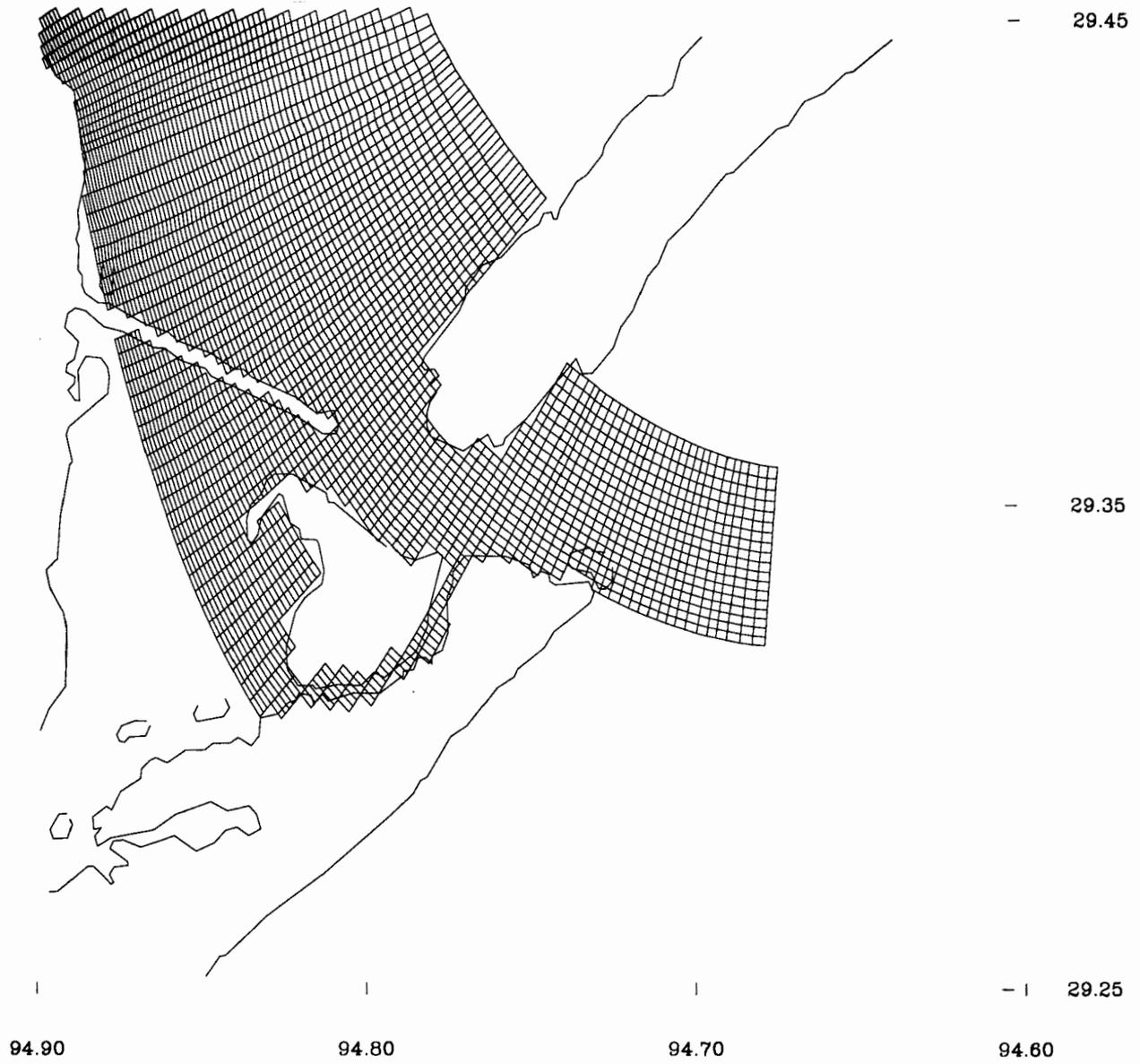
**Figure 2.8.** Houston Ship Channel Model Subgrid 1: Bay Entrance Section
