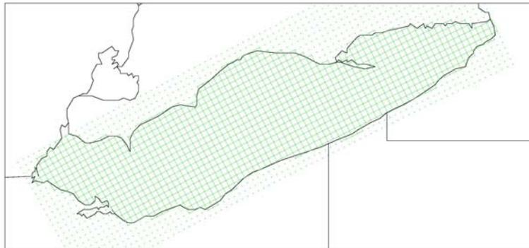
**Figure 2. Map depicting the POMGL grid domain with a grid increment of 5 km.**
