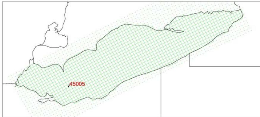
**Figure 6. Map depicting the location of the NWS/NDBC fixed buoy 45005 in Lake Erie along with the grid points of the GLOFS-Erie model grid.**
