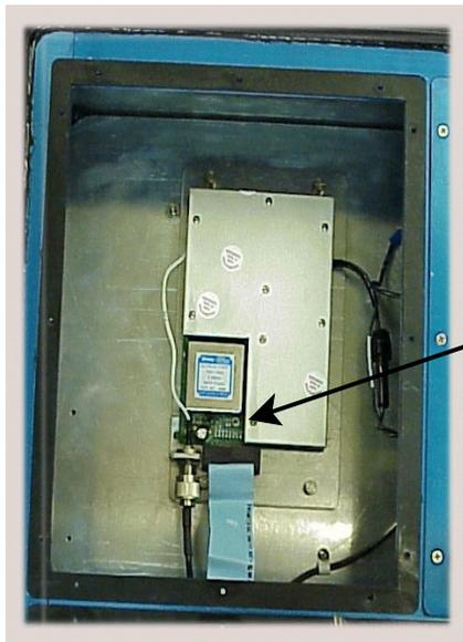
**Figure 10: GOES transmitter installed**
