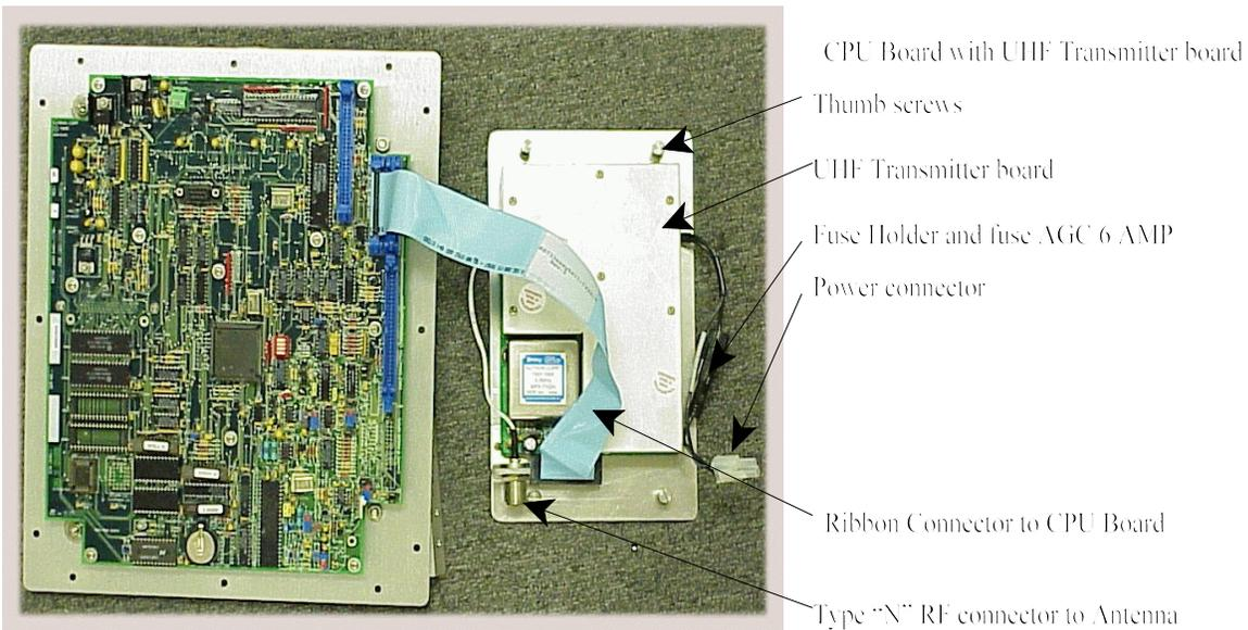
**Figure 9: GOES Transmitter and CPU Board**
