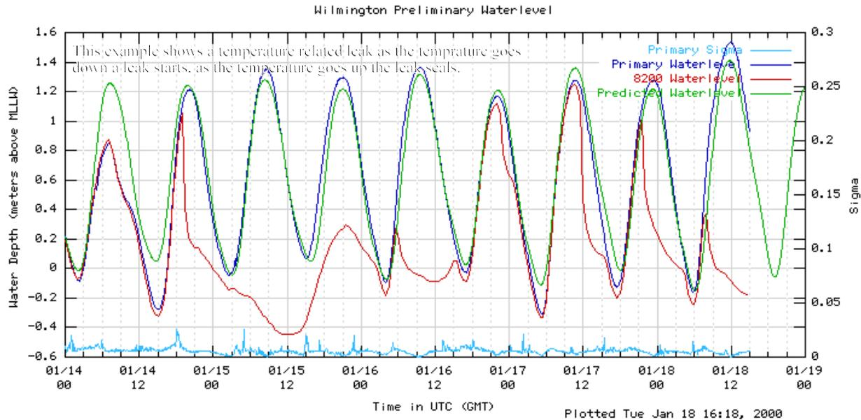
**Figure 14: Shows data graphs, of tidal data and temperature sensors taken from a NWLON primary tidal station.**
