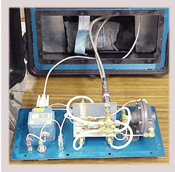
This Photo shows the Pressure control unit extended for leak testing note that the control unit has been twisted 180° to permit access to the fittings. Do not forget to check two fitting that are still inside the case at end of the medial braided hoses.
