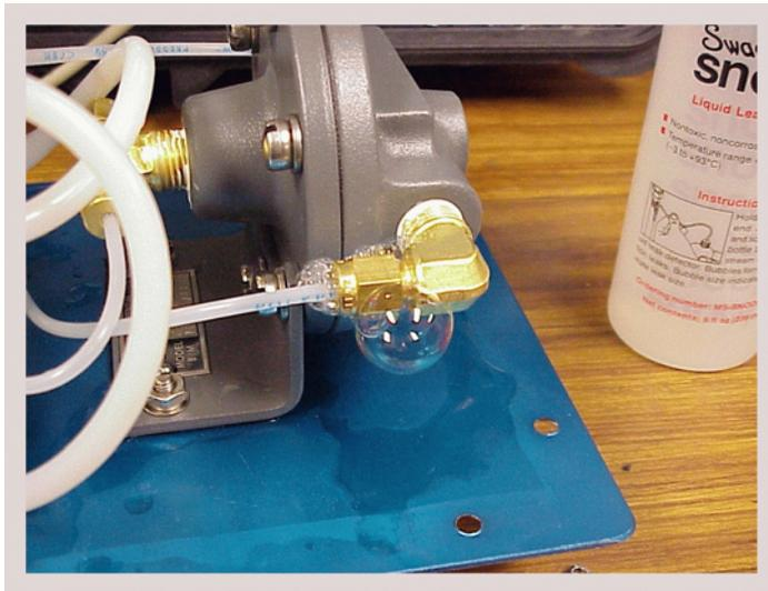
Note the bubbles forming around this fitting. Swagelok® "Snoop®" is a solution specially formulated to form bubbles around leaking fittings. A mix of one or two drops of Vicks Intensive Care hand lotion in a pint of water could be used if Snoop® is not available.
