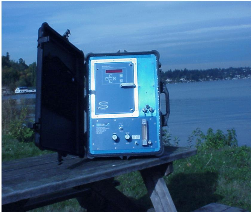
**Figure 1: 8210 Hydrographic Water Level Gauge**
