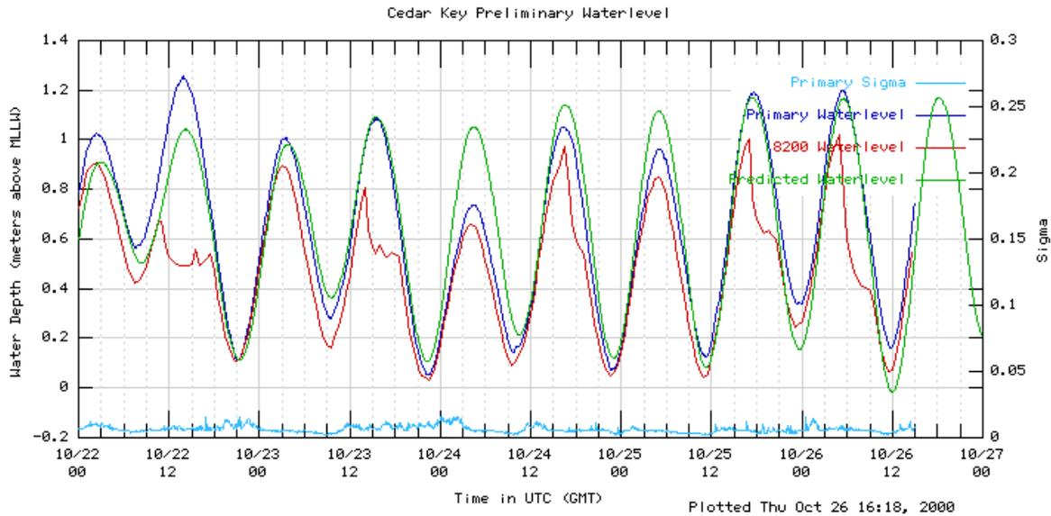
The Cedar Key data graph shows a leaking fitting probably in the manifold assembly. As the pressure increases the leak starts, and then pressure drops, and then as pressure builds again the leak opens again.
