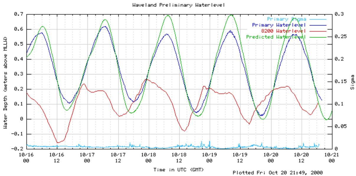
The Waveland water level example shows an tide station that has run out of gas notice how there is still a rise and fall of water levels but it dose not track the predicted and acoustic measurements.
