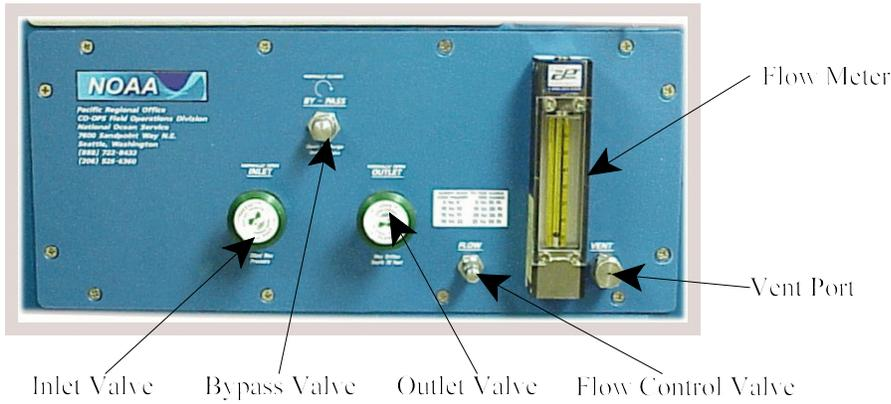
**Figure 5: Front of pressure control panel**
