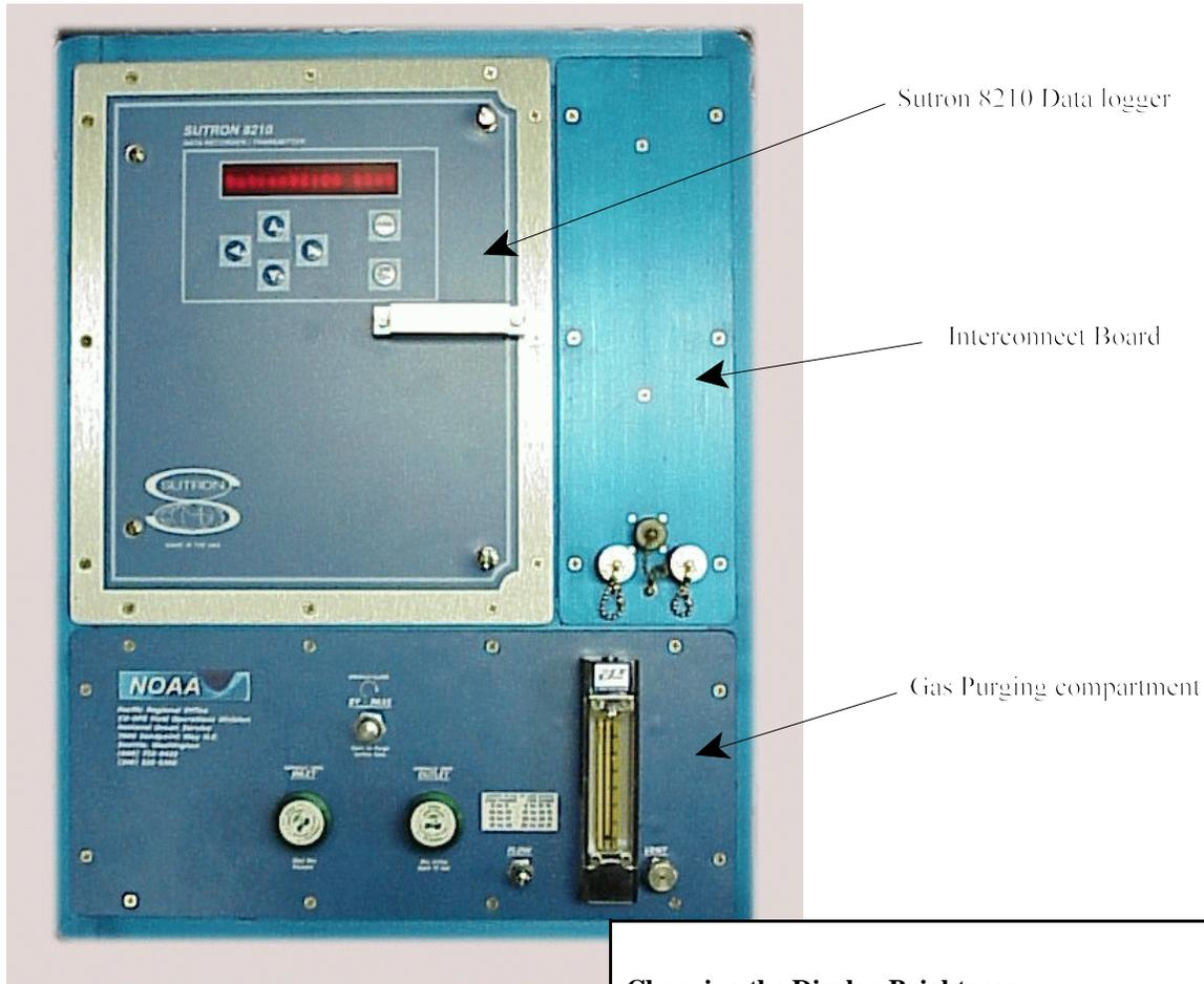
**Figure 2: Front Panel of 8210 Hydro Gauge**
