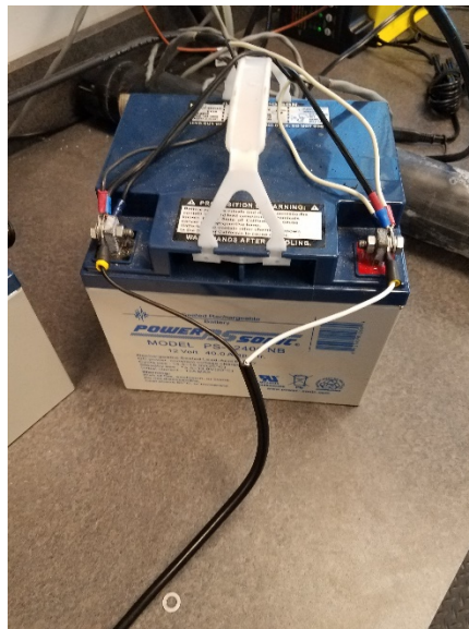
Figure 4. Circular crimps from voltage dividing cable have been connected to battery. Note that the pumpbox battery should typically have the following components already connected: Pumpbox power cable, IP power cable, & charging output cable from ASC solar voltage regulator
