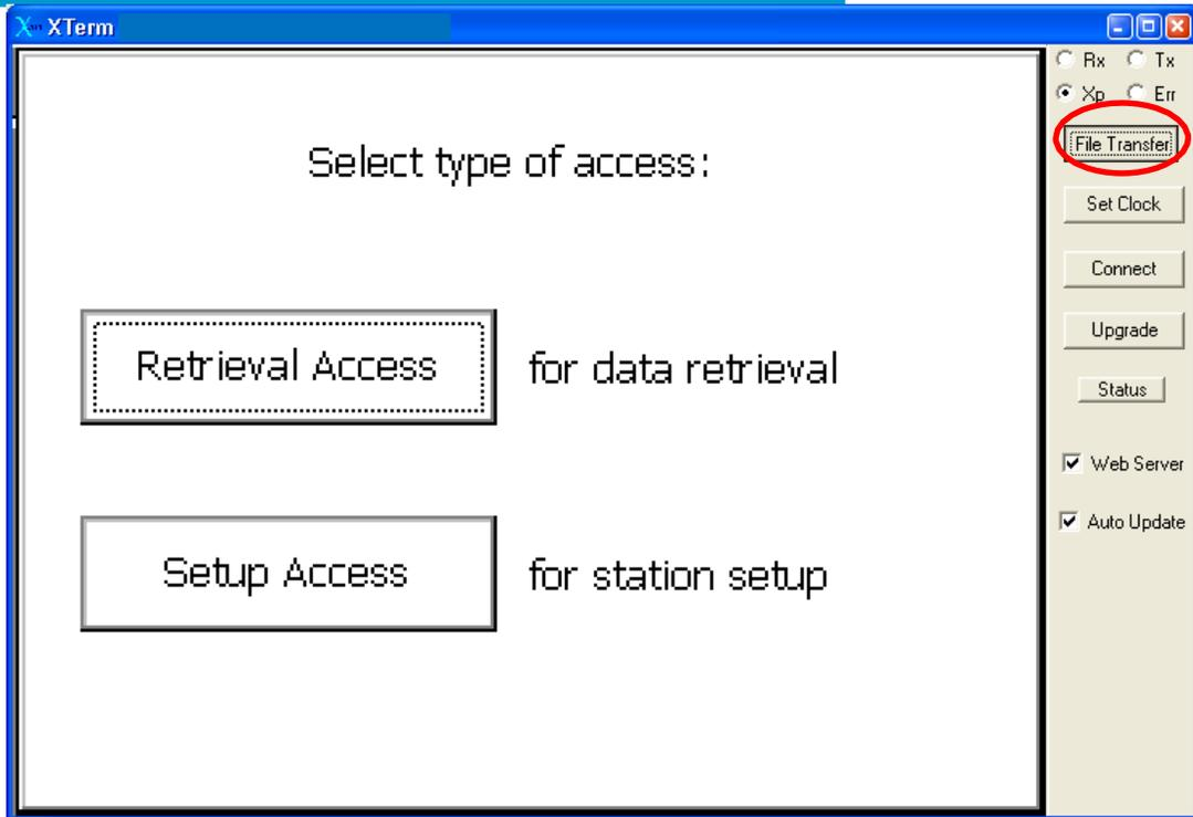
Navigate to the "Extra SLLs" directory on your local hard drive and select NOS.SLL to transfer to the Xpert2. ***(NOTE: Some installations will require the upload of other SLL files as needed, CIL will specify the stations where this is necessary)***
