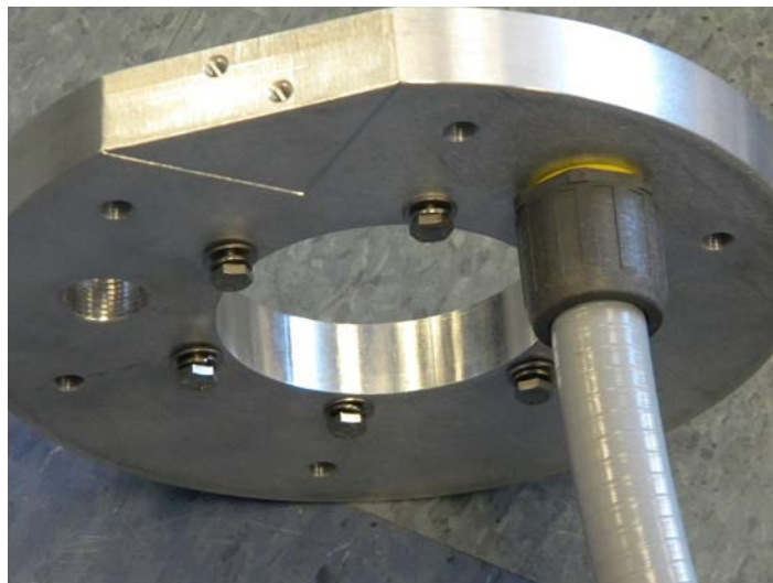
Figure 3-8. Cable run through hole in collar with Liquid-tight conduit attached from below.
