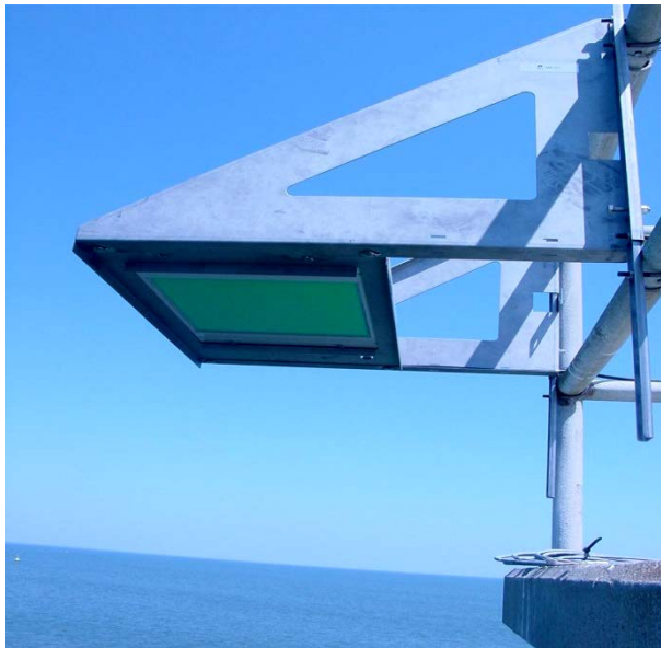
Figure 2-1. Miros Microwave RangeFinder.
