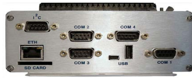
Figure 2-4. Sutron Xpert 9210B DCP I/O/ modules
