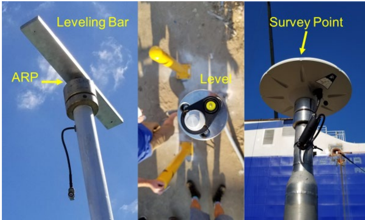
Figure 4. The left photo shows the level bar used to measure to the ARP, the center photo is the bubble level to ensure the SA is level, and the photo on the right shows the ZG survey points.
