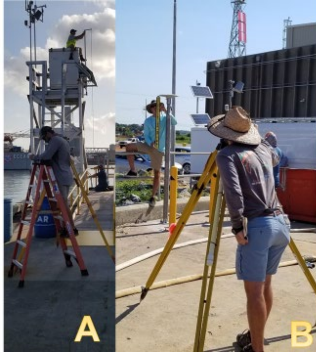
Figure 5. Photo A uses a tape down method and photo B uses a leveling rod.
