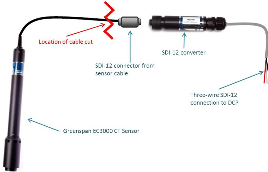
Figure 2-6. Greenspan EC3000 sensor cabling; red line shows where cable will be cut.
