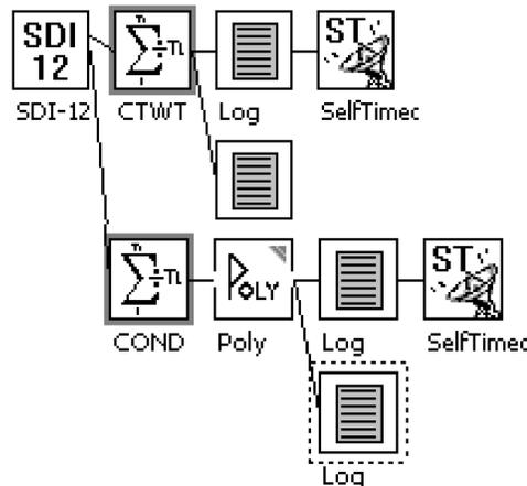
**Figure 3-8.** Final graphical setup for a Greenspan CT sensor, which is configured by CIL/SIL prior to deployment.
