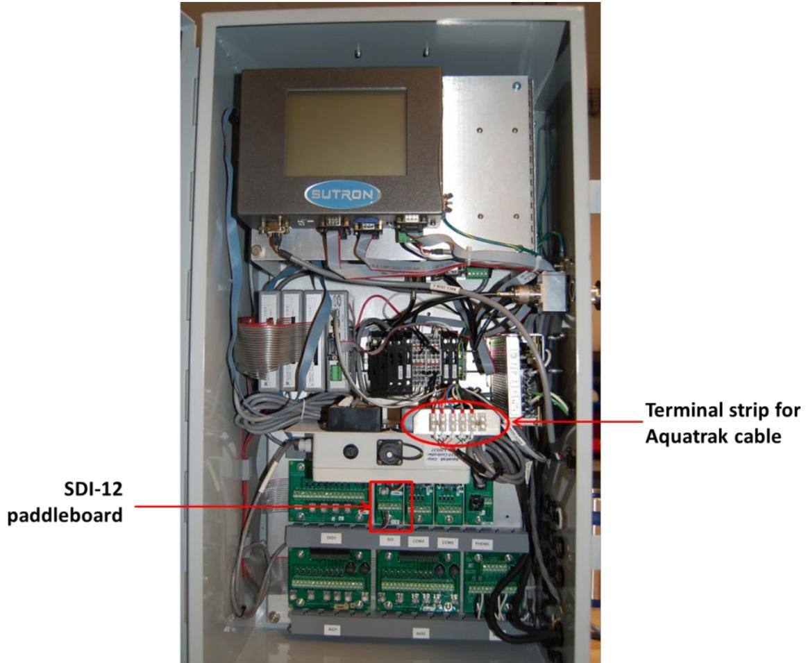
**Figure 3-1.** Typical CO-OPS system with Aquatrak controller
