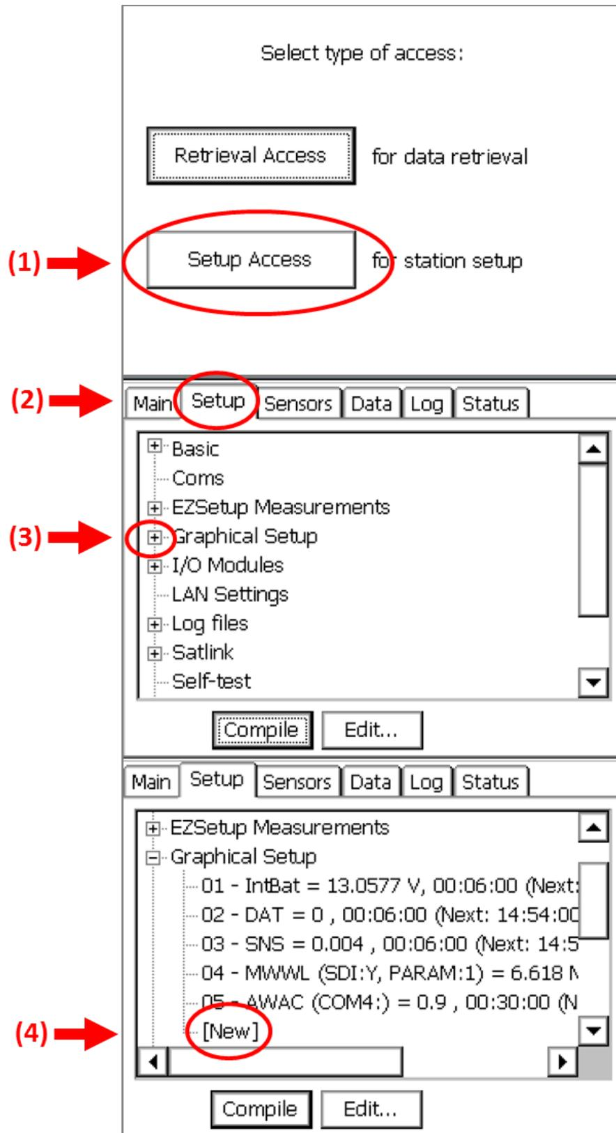
Figure A-1. Add a new graphical setup.
