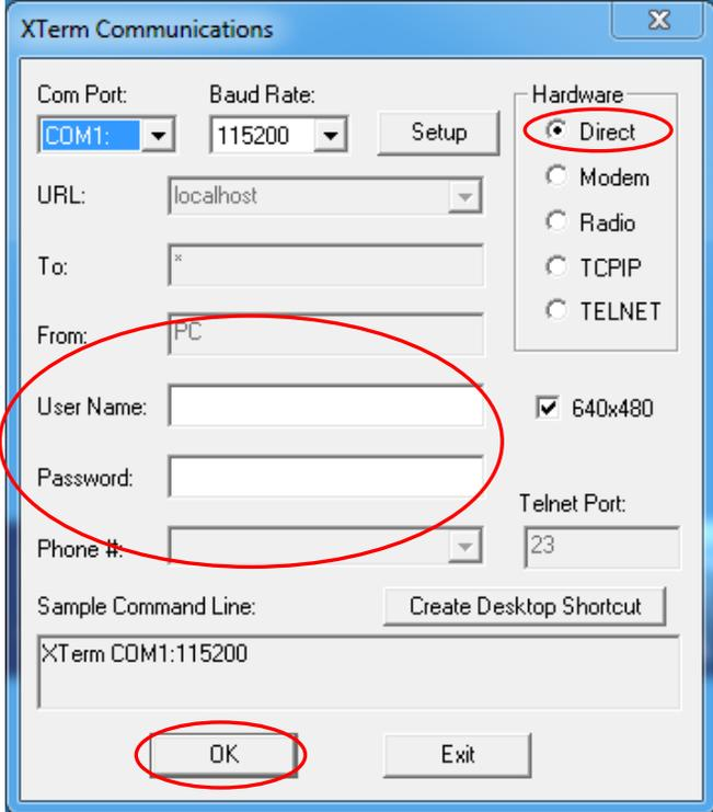
Figure 3-5. Xpert connect screen.
