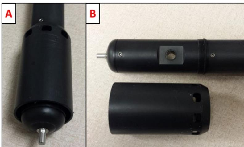
**Figure 2-2.** Greenspan EC300 CT Sensor with A) shroud in place and B) shroud removed.
