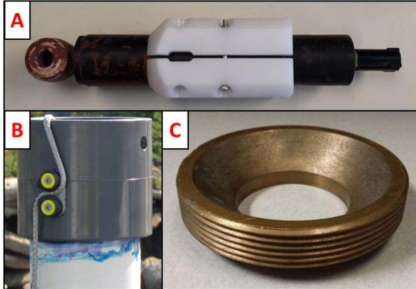
**Figure 2-3.** A) FSI CT sensor housed in Delrin® clamp. B) The top of a CT well showing locking mechanism for line/pulley system. C) The brass collar that catches the Delrin® clamp at base of well.
