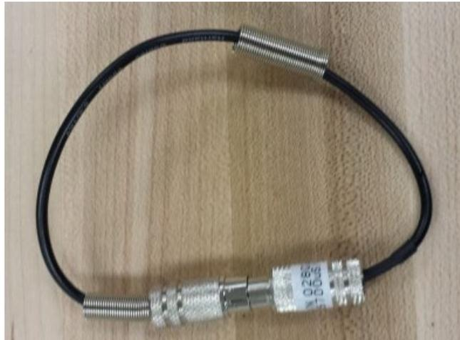
Figure 2-4. Loop calibrator
